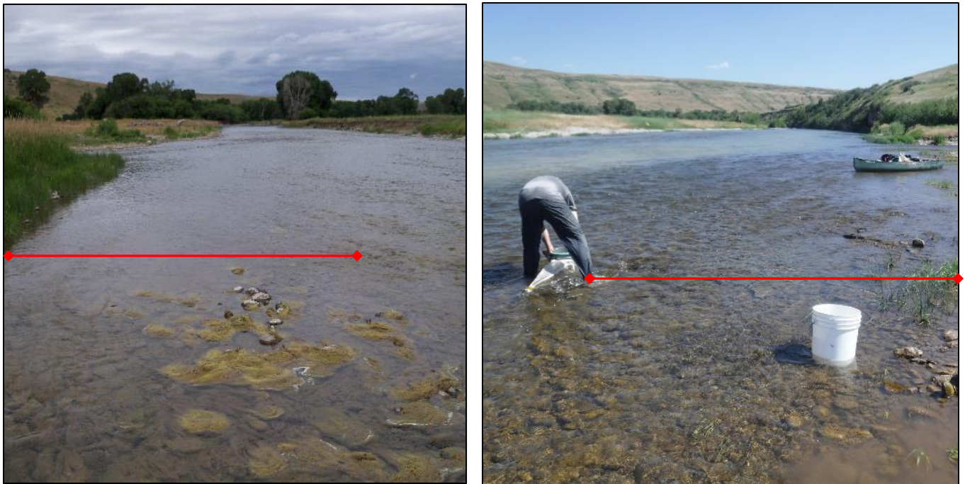
Photo 2. Hess sampling procedure in the Smith River near Hound Creek confluence (BKK133) in 2016 (l) and 2018 (r). Distance from the greenline to the sampler was measured (redline).
