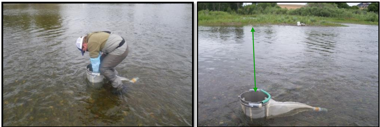
Photo 1. Hess sampling procedure in a Missouri River riffle near Little Prickly Pear Creek (MO_LPPC_US). Distance to the greenline was measured.
