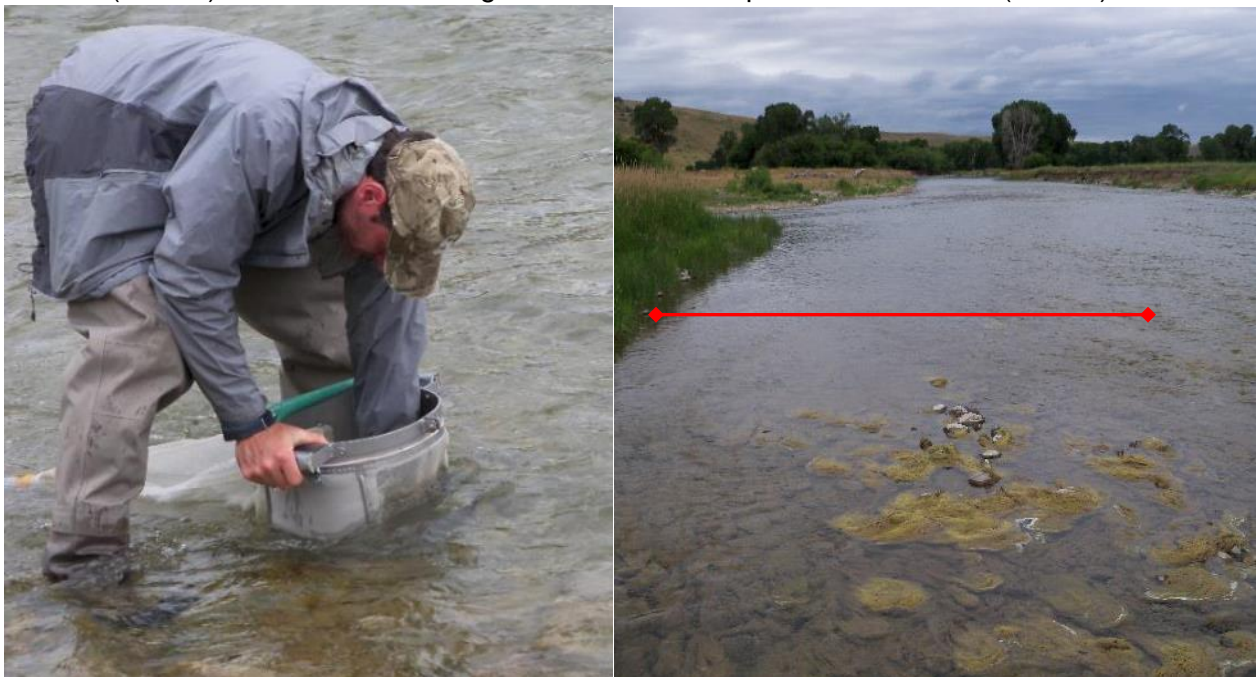
Photo 1. Hess sampling procedure in a Smith River riffle near Hound Creek confluence (BK133). Distance from the greenline to the sampler was measured (redline).
